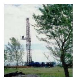
Rig is designed for: - drilling, workover, examination and servicing wells
