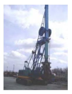
Crane is designed for: - excavation of diaphragm wall panels up to 40 m in gravel, clay, sand
